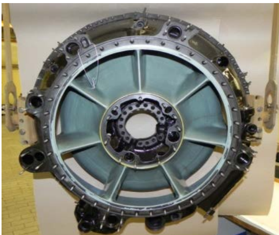
Turbine intermediate casing with anti-corrosion coating
